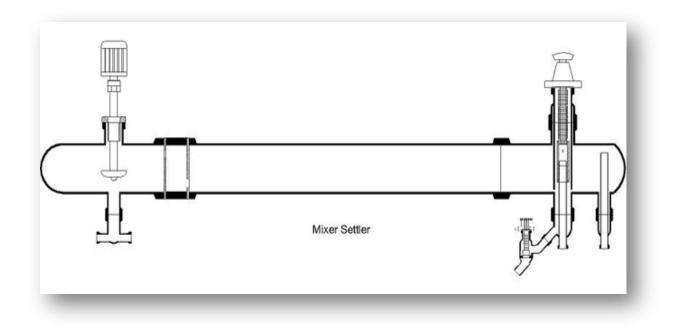
By connecting several mixer settler stages in service and arranging for the phases to flow counter current to each other, the plant can be adapted to handle the particular separation problem in hand.
