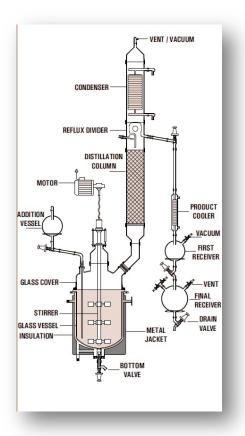
According to the customer's requirements and standard, we manufacture jacketed glass reactor which has many functions to satisfy kinds of experiments. Goel Scientific offers Glass Reactor with Metal Jacket for chemical & pharmaceutical industries for process development. Glass reactor will have metal jacket and metal insulation.
