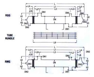
Dimensional Specifications of Shell and Tube Heat Exchanger :
